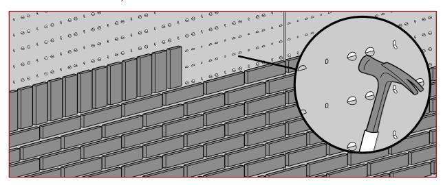
Thin brick veneers should be stopped 3/8 in. from door and window trims.
