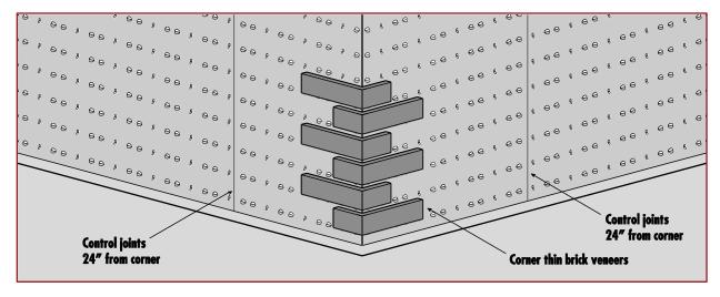
3. Install one row of thin brick veneer the length of the wall to the next outside or inside corner. Whenever possible, the master row should go under or over windows or door lines with a 3/8 in. joint opening between thin brick veneers.
