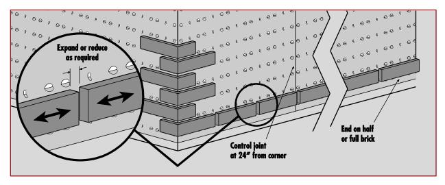
4. The position of the thin brick veneer on the panel tabs will be the same on every other course. Tabs can be bent up or down to adjust brick alignment, as required.
