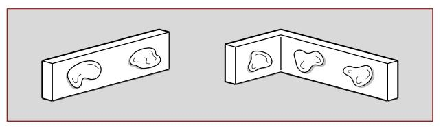
Vent mastic by pulling thin brick veneer away from panel for a few seconds. Then push back into place. This allows solvent to escape faster and the mastic to become stickier.
